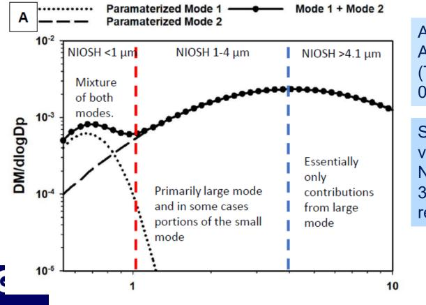
Aerosol size distribution: Aerodynamic Particle Sizer (TSI APS 3321) 0.542- 20 µm, 52 size bins
